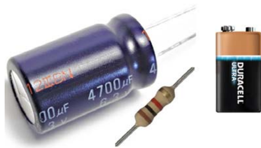
Figure 2 Electrolytic Capacitor ( 4'700 \mu\text{F} ), Resistor ( 1'000 \Omega ) and Battery (9 Volt)
