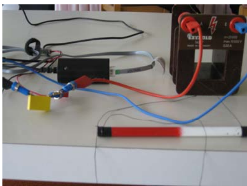
Figure 15 Coil (23'000 turns), Bar Magnet, R-C-Filter and EasyLink Adapter
