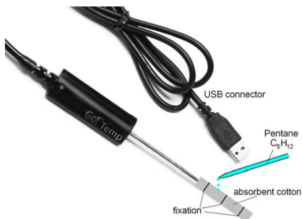
Figure 6 Measuring the Evaporation Heat of C_5H_{12} from an absorbent Cotton Ball on a GoTemp/EasyTemp Sensor
