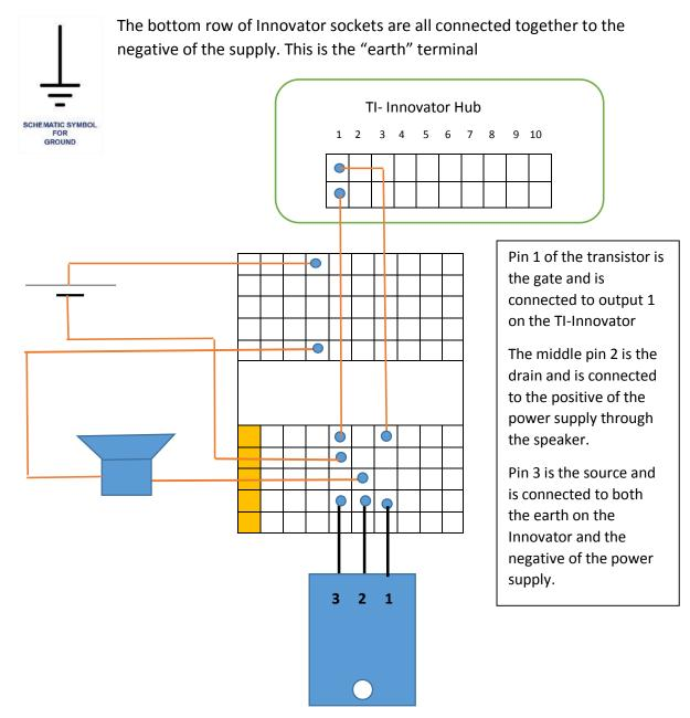
The transistor used, <u>Z34N</u>, is shown with the front containing the writing facing upwards. It is a MOSFET power transistor able to handle currents of 10 A. The pin functions arev described above.
